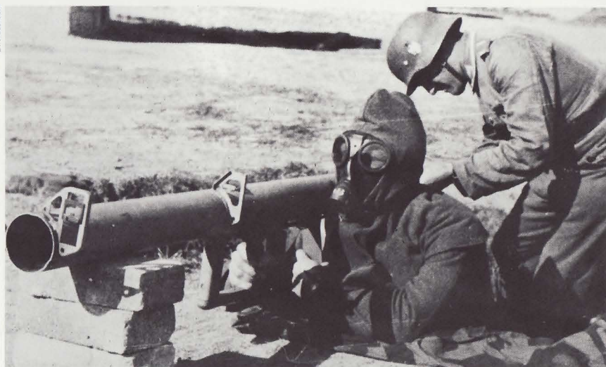
The blow-back of the Raketenpanzerbüchse 43 without protective shield was so great that the operator was to wear protective clothing. As an improvisation he could wear his gas mask without filter, a hood using his gas cape, a scarf, and gauntlets.
